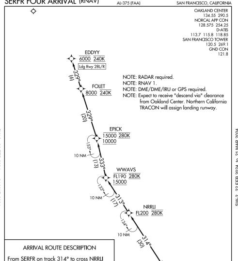
at or above FL200 and at 280K, then on track 313° to cross WWAVS between 15000 and FL190 and at 280K, then on track 333° to cross EPICK between 10000 and 15000 and at 280K, then on track 329° to cross FOLET at or above 8000 and at 240K, then on track 329° to cross EDDYY at 6000 and at 240K. Expect assigned instrument approach (Rwy 28L/R).
